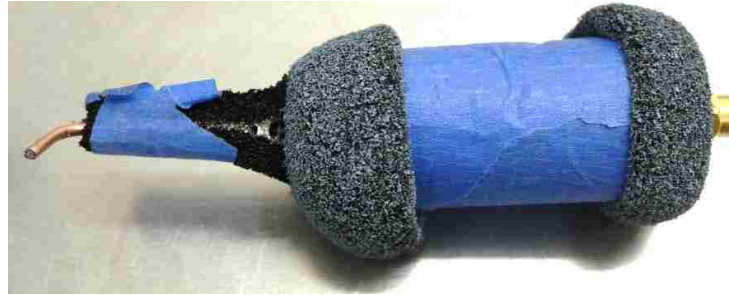
Figure 1.34. E field probe used for the near field scanning setup.
