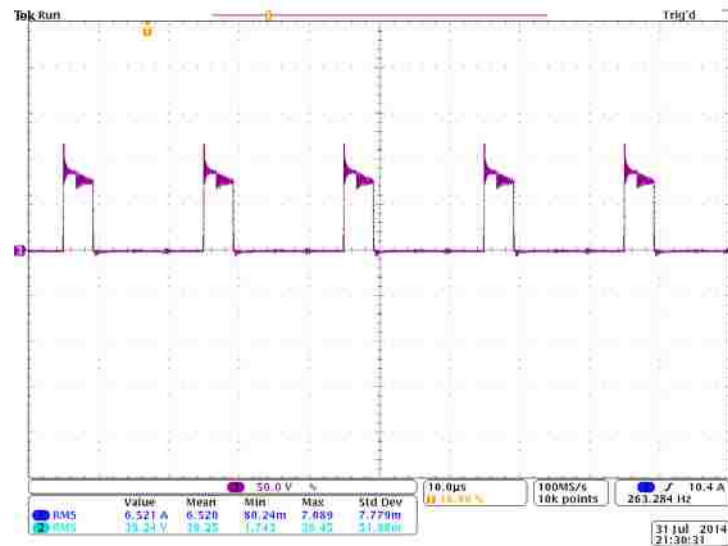
Figure 4.9 Drain-source voltage stress on S_1 of interleaved boost converter in [6]
