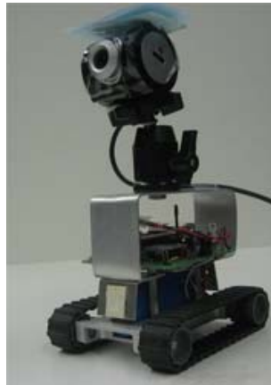
Figure 2.8. Follower Robot Fitted With a CCD USB Camera.
