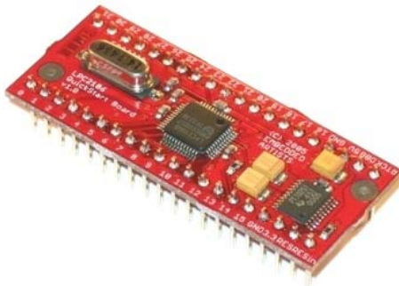
Figure 2.3. The ARM7 LPC2106 Controller from Philips.
