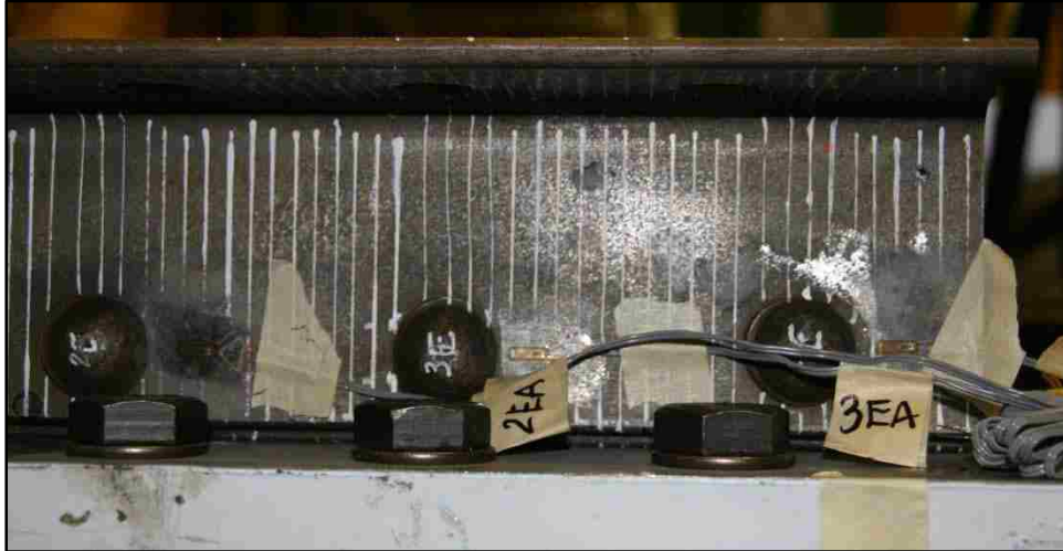
Figure 3.40 Strain Gauge Placement on East Angle
