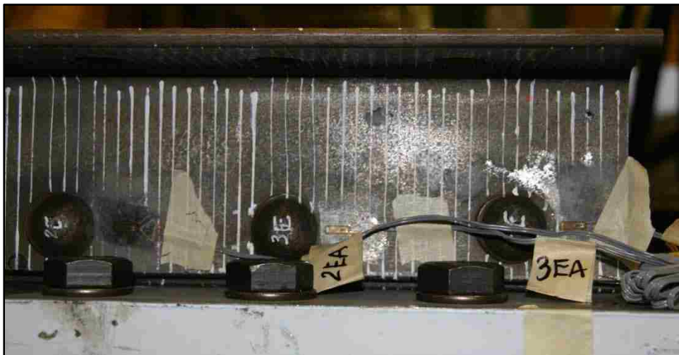
Figure 3.40 Strain Gauge Placement on East Angle
