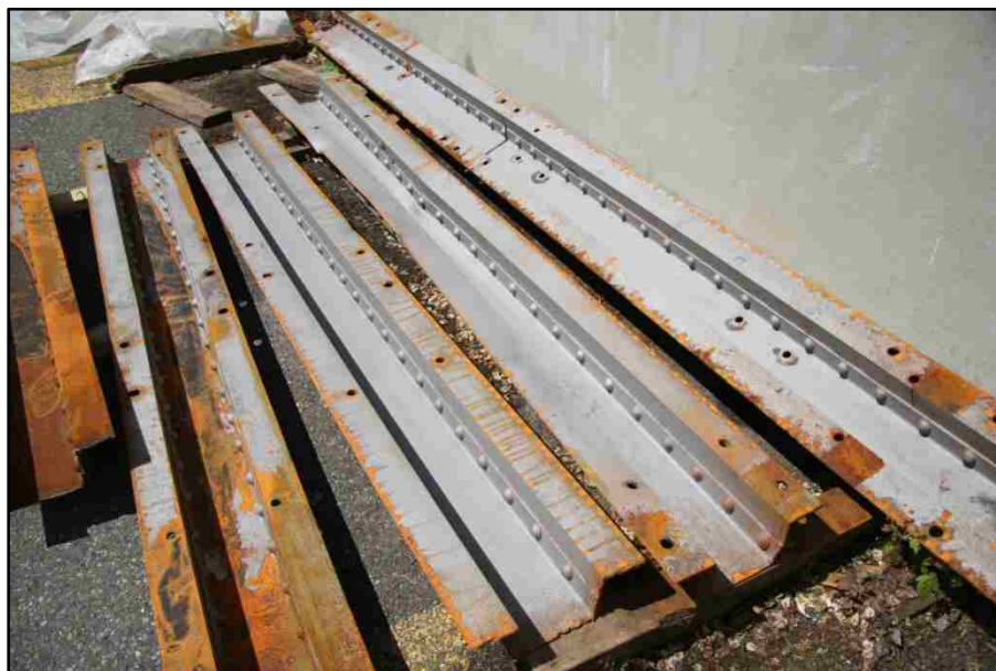
Figure 3.8 Guardrail Specimens after Sandblasting
