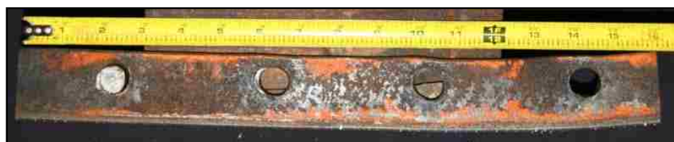
(a) East Channel Flange Faying Surface
