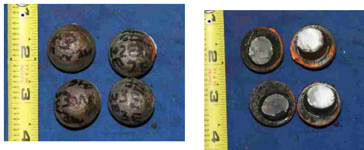
Figure 4.40 Fractured Rivets - Specimen 2R (4L)
