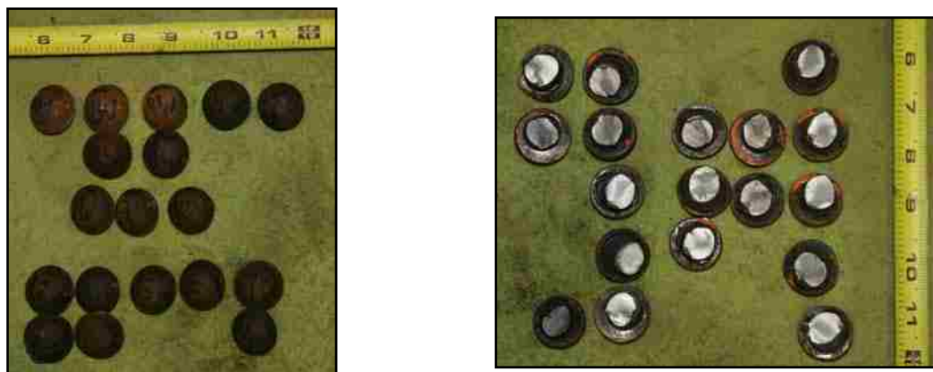
Figure 4.66 West Guardrail Fractured Rivets – Specimen 17R
