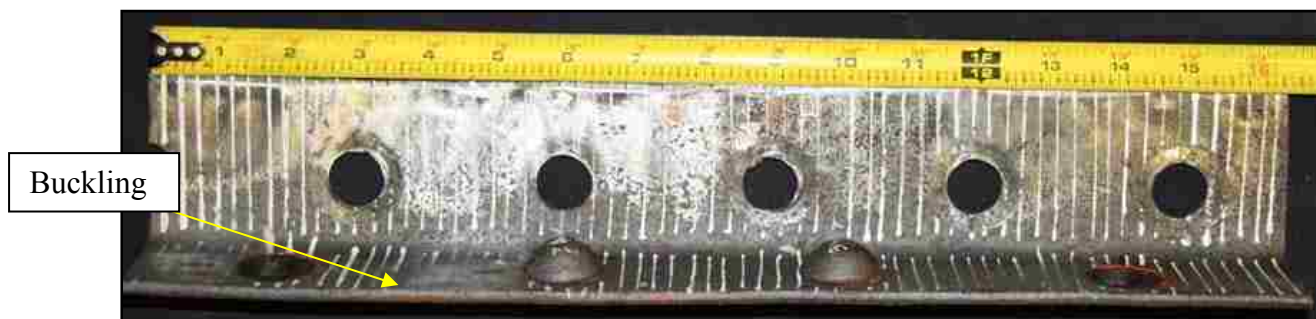
Figure 4.21 West Channel Buckling – Specimen 4R
