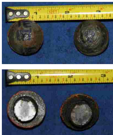
Figure 4.32 Test 2R Fractured Rivets
