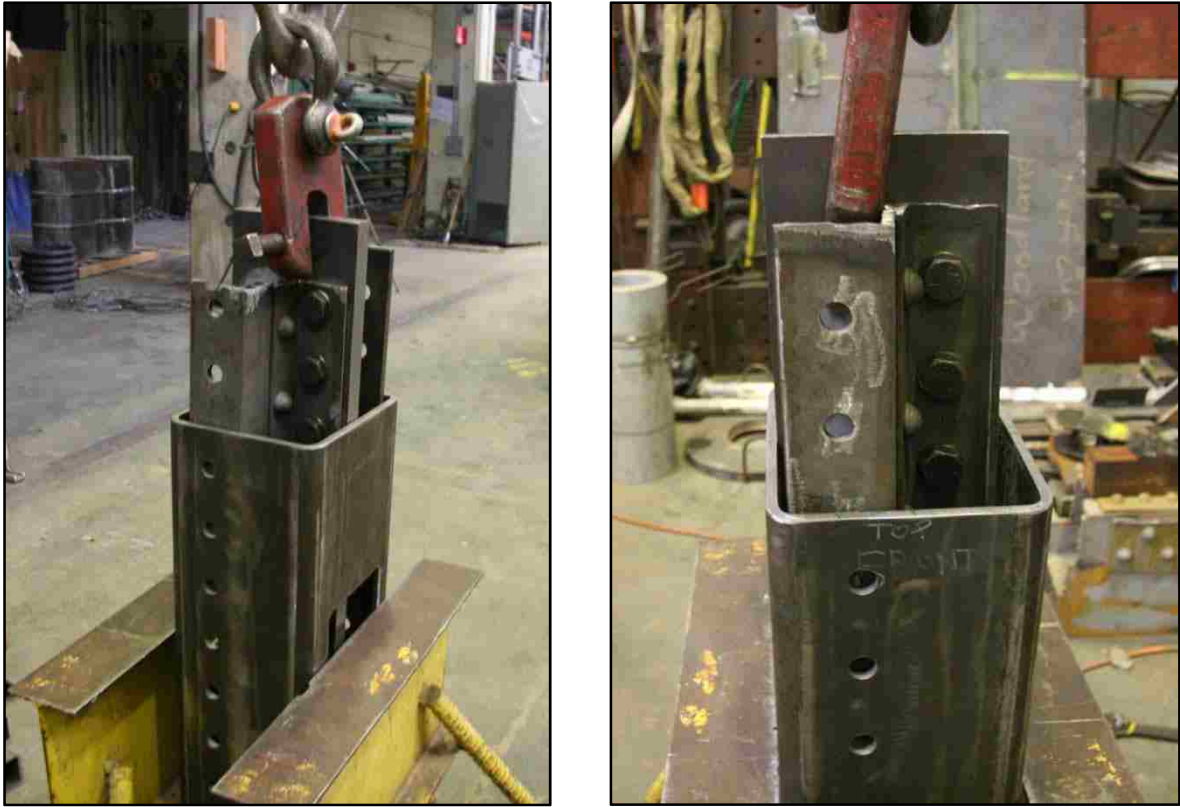
Figure 3.41 Assembly of Plate, Guardrail, HSS (a) East Guardrail (b) West Guardrail
