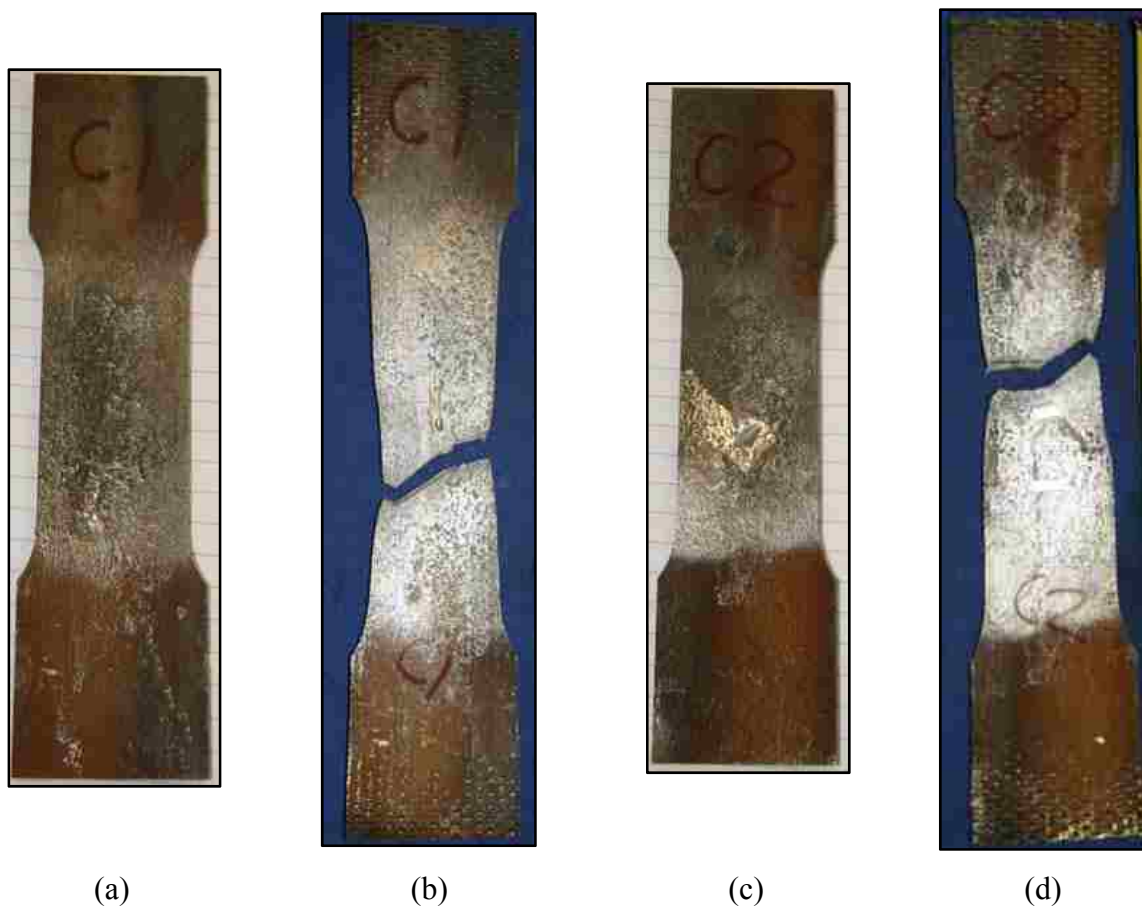
Figure 4.4 Channel Coupons Tension Testing (a) C1 before (b) C1 after (c) C2 before (d) C2 after
