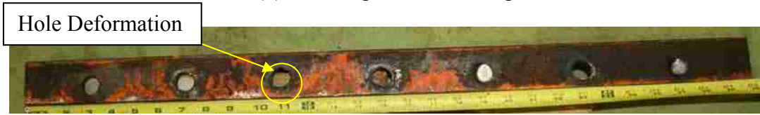
(c) East Channel After Testing
