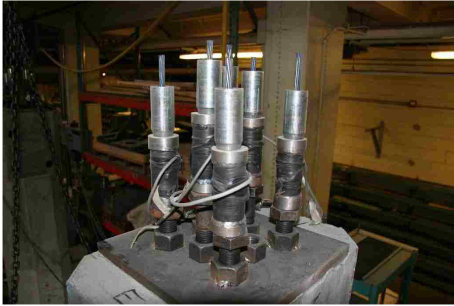
Figure 3-5: System of STD, strand load cells and strand chucks on top of one specimen.
