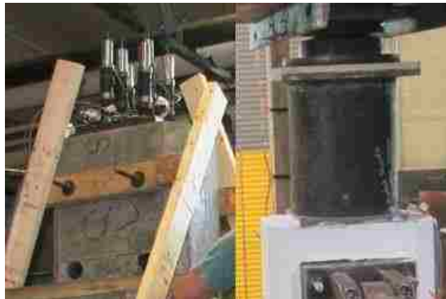
Figure 3-2: Strand slip detecting setup (left) and the setup covered by the vertical loading device (right).
