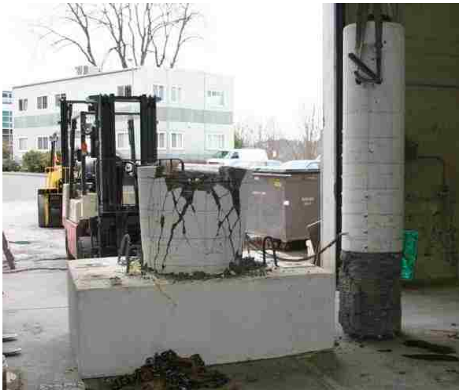
Figure 4-3. Specimen DS-2 after testing
