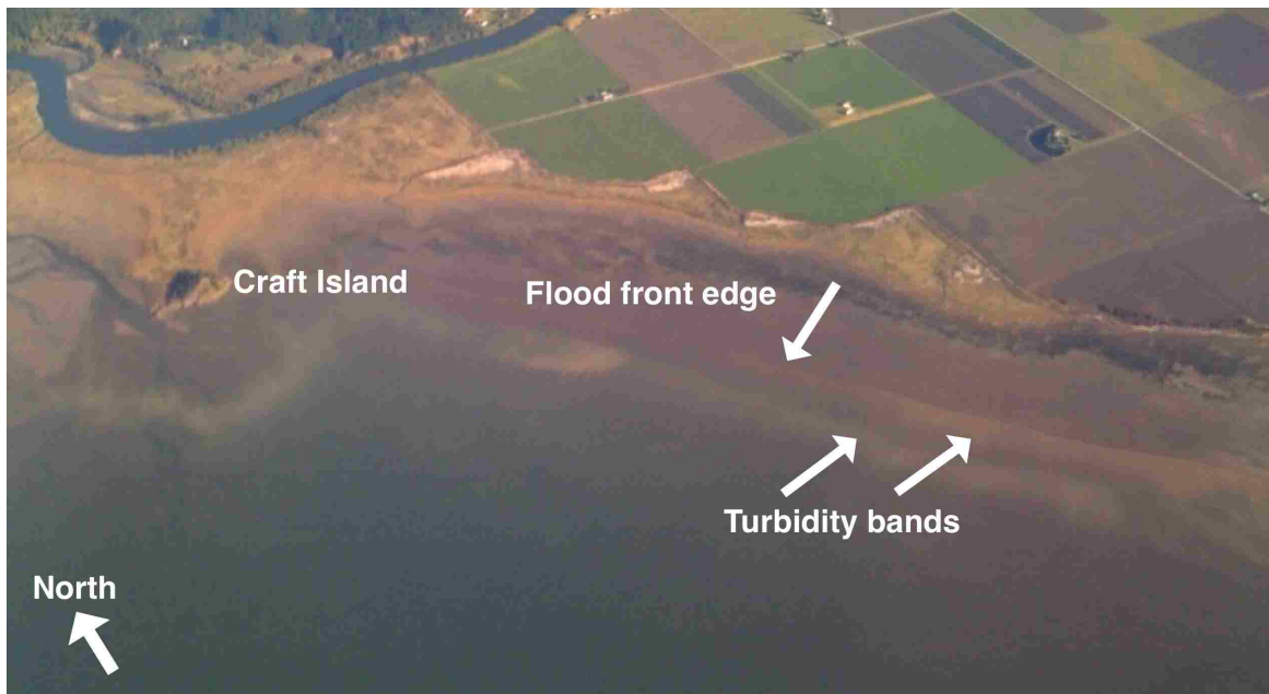
Figure 4.11 Oblique aerial photograph of North Skagit Bay showing turbid water near the flooding front. Two bands of turbidity associated with the edge of the front are indicated.
