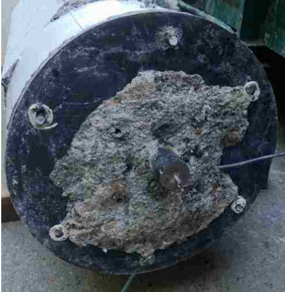
Figure C.6 Bottom of shoe after testing.
