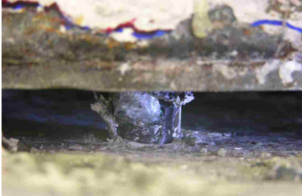
Figure 4.9 Exposed north bar of PreT-SF-ROCK.
