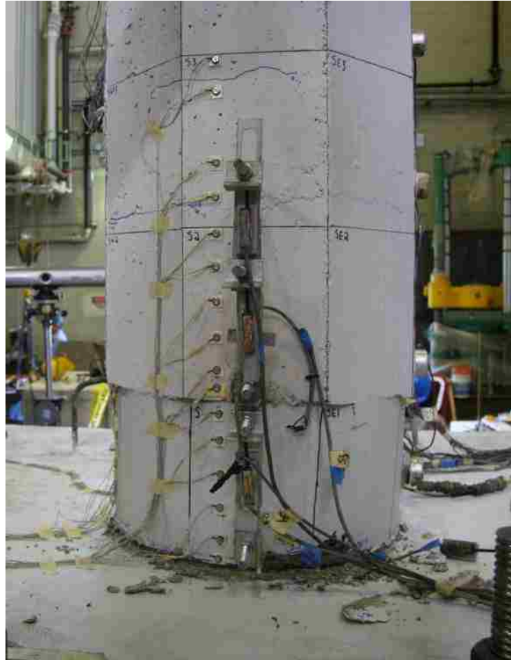
Figure C.1 South view after 6% drift, cycle 9-1.
