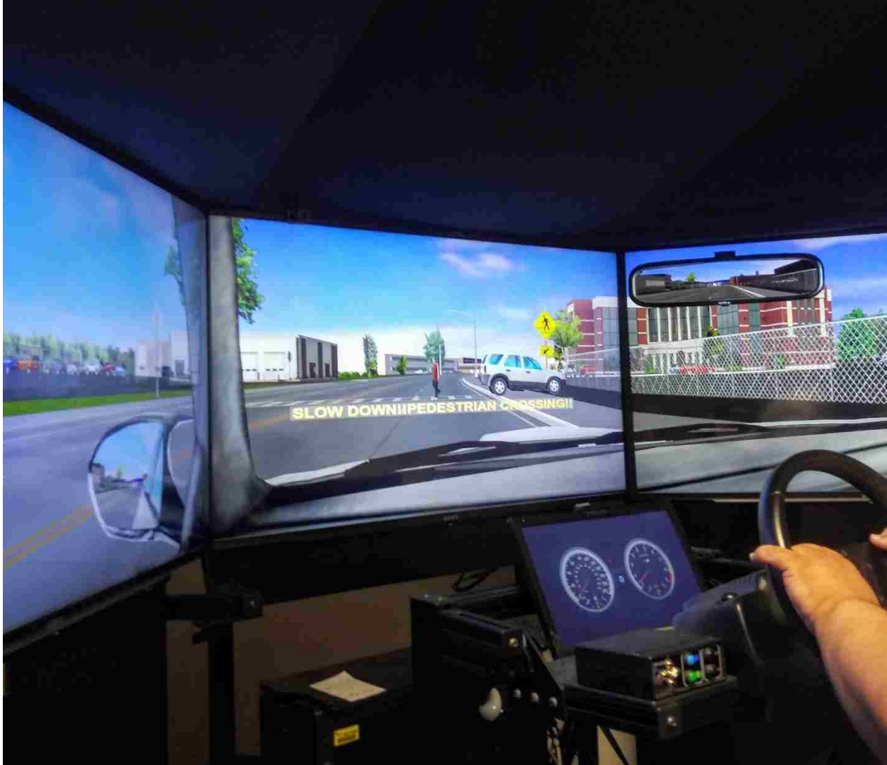
Figure 12. NADS MiniSIM driving simulator with HUD interface
