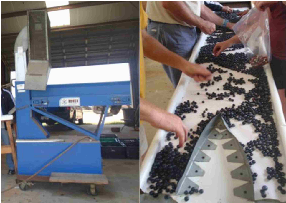
Figure 3.10. Stalk separator (left) and the procedure of separating the branches and leaves from the fruits.
