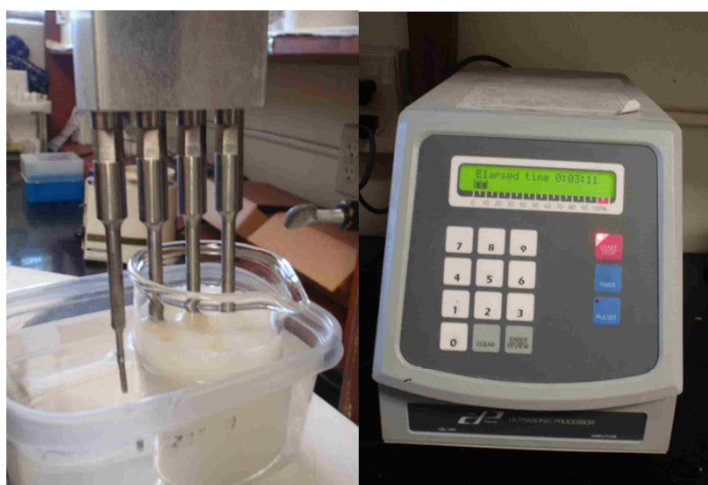
Figure 3.15. Preparing salmon oil-in-water emulsion by using sonication.
