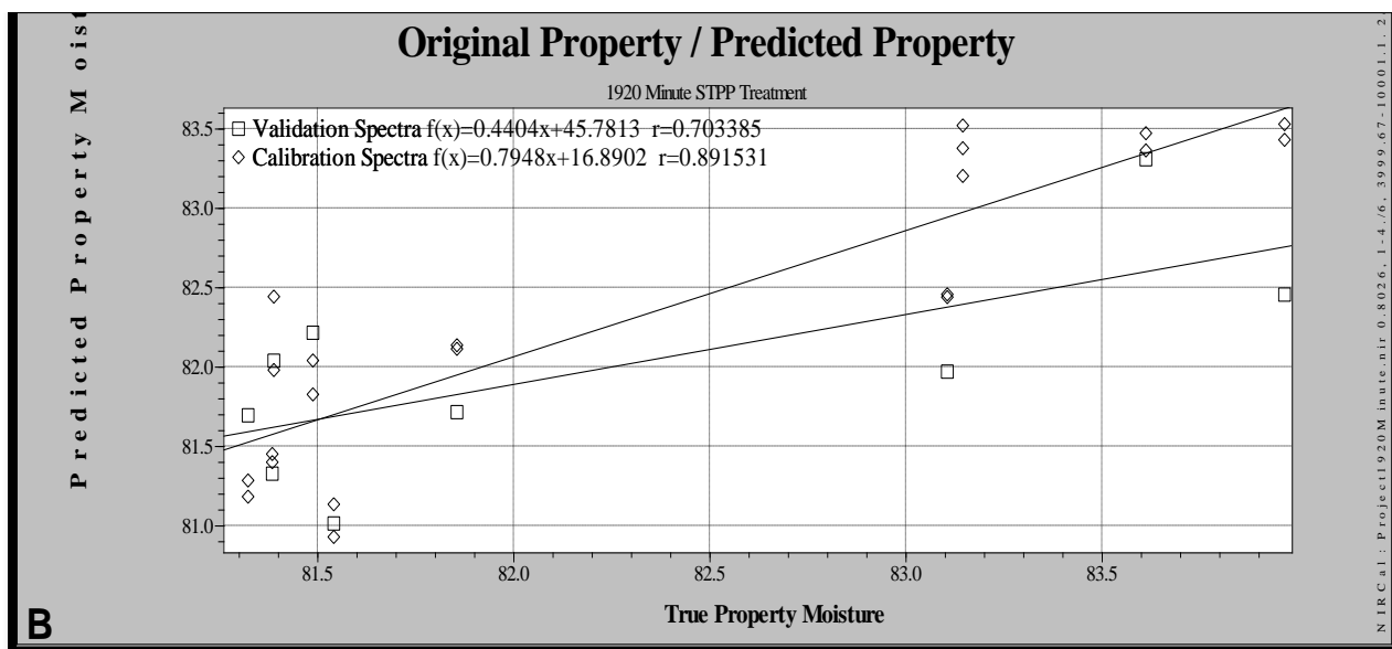
Figure 21 – A plot of the original property against the predicted the predicted property for the partial least squares regression for the 1920 minute treatment.
