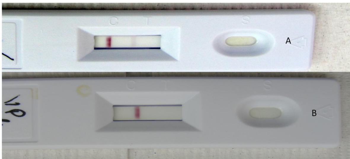
Fig. 5.2. Test strips. V. vulnificus ATCC 27562 bacterial suspension 10^4 CFU/ml (A) and (B) V. parahaemolyticus were applied to the test strips. T = test line; C= control line.
