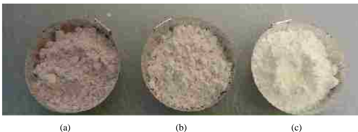
Figure 3.8 Image of microencapsulated 10MMOBJ, 5MMOBJ and MMO powders (a, b, and c respectively).
