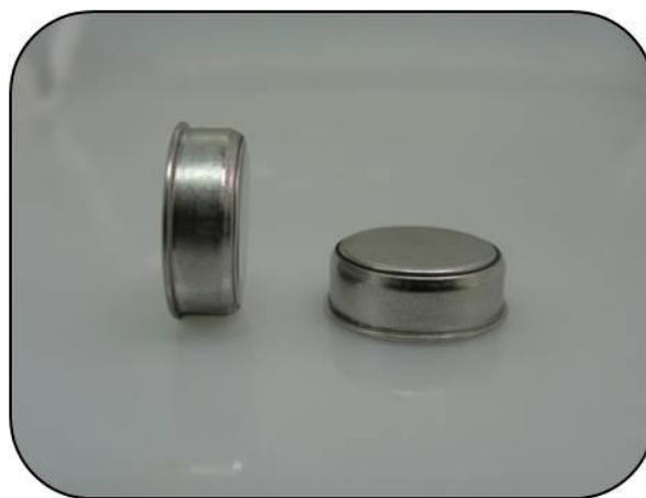
Figure 5: Side and front view of an ACR SmartButton® temperature data logger.
