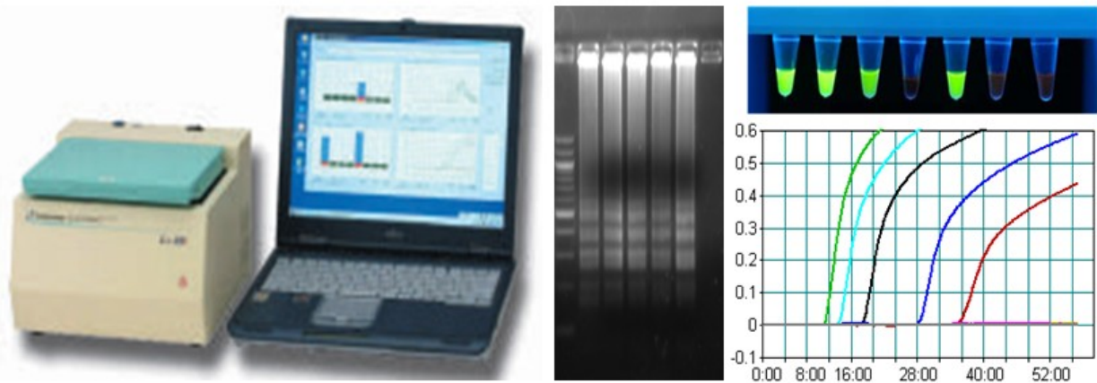
FIGURE 2.7. Loop-mediated isothermal amplification turbidimeter and three result observation methods.
