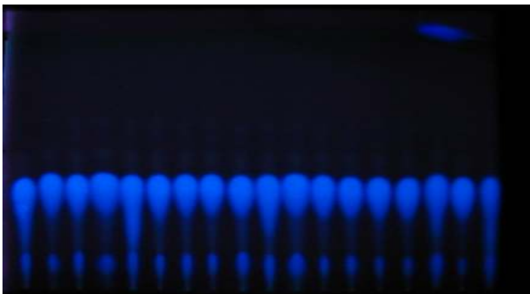
Figure 4.19. Thin layer chromatogram of relatively purified [^{14}\text{C}]\text{-AFB1} . No standard aflatoxins are shown.
