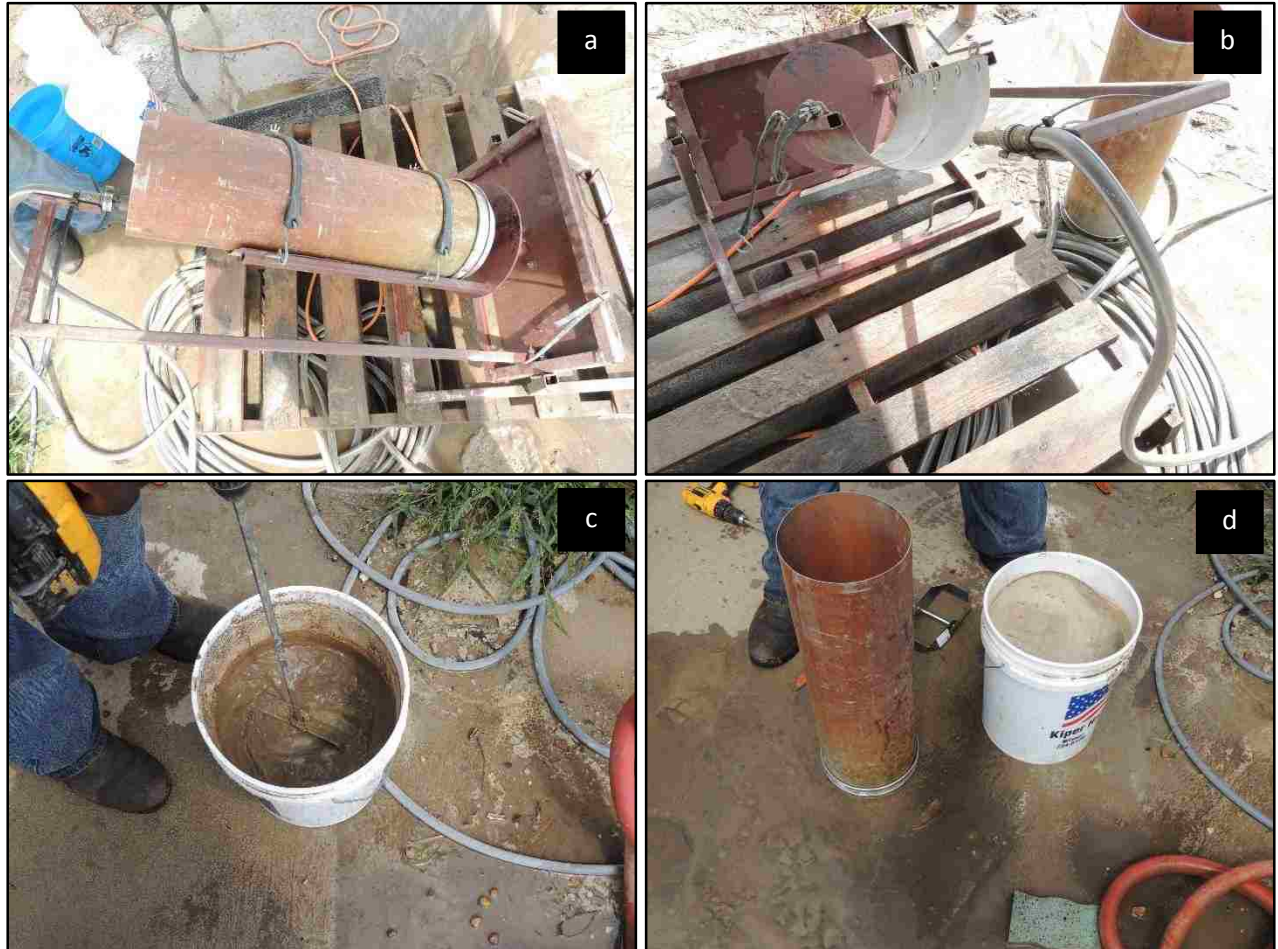
Figure 3.4 (a,b) Water-spray system used to extract prickly sida seed from soil; (c) aluminum pipe and sieve; and (d) drill and wall mixer used in preparing soil slurry.
