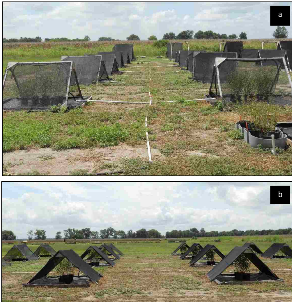
Figure 3.1. (a) A-frame shade structures showing watering system and wooden boxes used to catch seed; and (b) side view.
