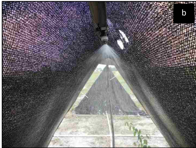
Figure 3.2. (a) Water trailer used for water supply; (b) two brass \frac{1}{2} HH 30WSQ FullJet nozzles; and (c) prickly sida pots shortly after watering.
