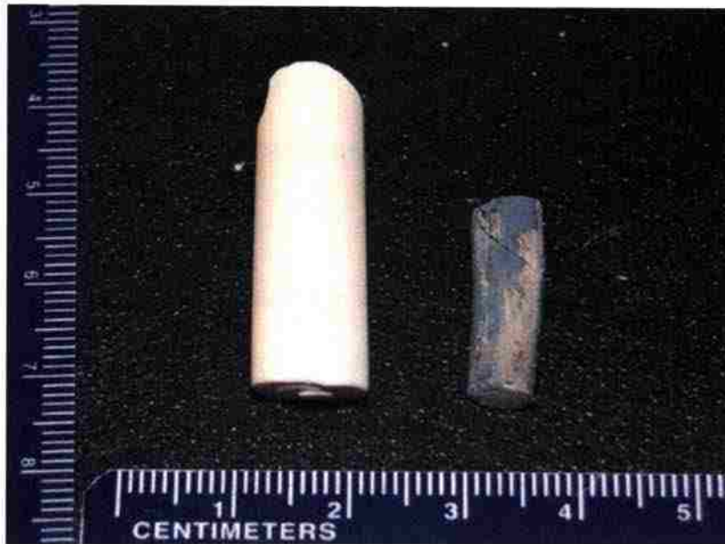
Figure 10. Photographs of a F-20-45 PAN-crosslinked silica aerogel (left), and of the resulting SiC aerogel (right) after (a) aromatization (225 °C in air); (b) carbothermal reduction (1400 °C under flowing Ar); and (c) oxidative removal of unreacted carbon (600 °C in air).
