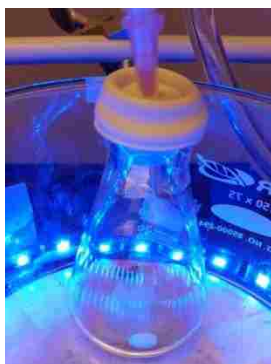
Figure 5. Grafting Setup with Stirbar, BNAH, and Template-Stripped Gold Substrate in Preparation. This setup was used for particle lithography experiments.
