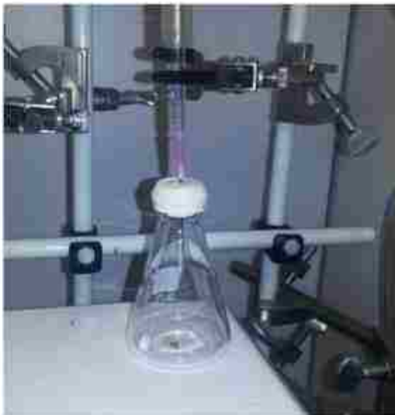
Figure 2. Photograph of the apparatus used for immersion of gold substrates. The substrate is located at the center bottom area of the flask. The stir bar rotates at the side of the flask.
