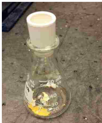
Figure 5. Grafting Setup with Stirbar, BNAH, and Template-Stripped Gold Substrate in Preparation. This setup was used for particle lithography experiments.
