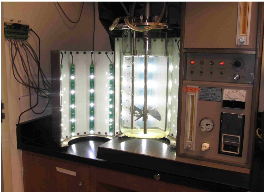
Supplemental figure 1: 15L photobioreactor with LED lighting.
