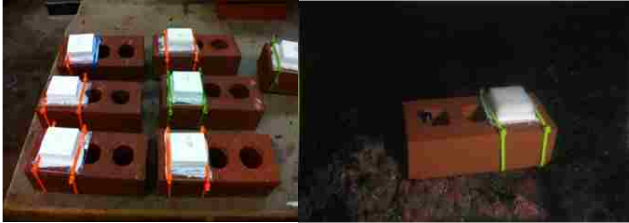
Figure 2. Completed alabaster dissolution block assembly, above and below the waterline.
