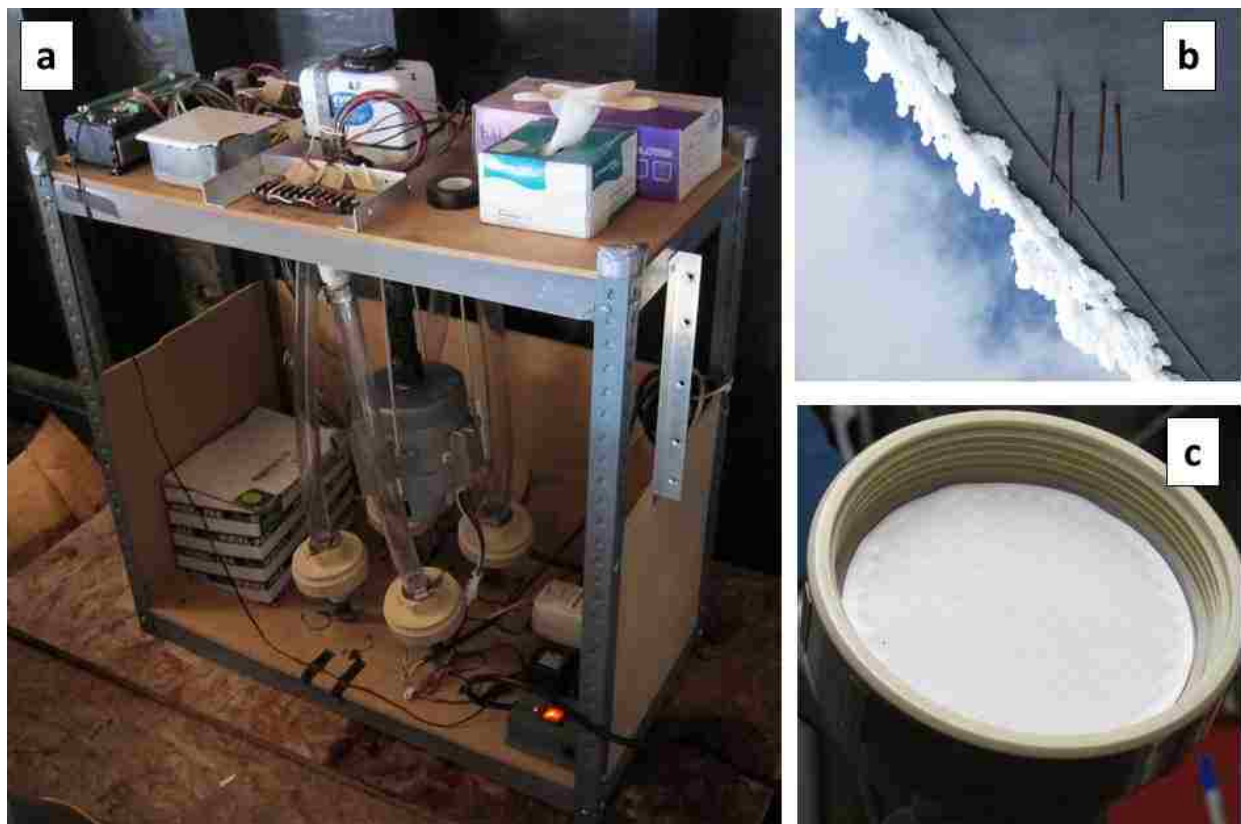
Figure 2.1 Air sampling apparatus at the Mt. Bachelor Observatory. (a) A high vacuum pump, electronics board and 4 separate filter housings were connected to intake pipes through holes at the base of the device. (b) Copper intake pipes emerged outside the building, facing into prevailing winds. (c) Polyethersulfone filter membrane (254 cm 2 , 0.8 µm pores) inside plastic housing after sampling period.
