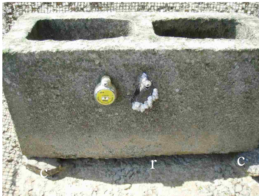
Fig. S3. Side view from east of one plot. Cobble spacers (c) provide shaded crack refuge (r) approximately 25 mm in height beneath cinder block
