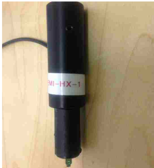
Figure 3.1. H-field probe used for hand scanning
