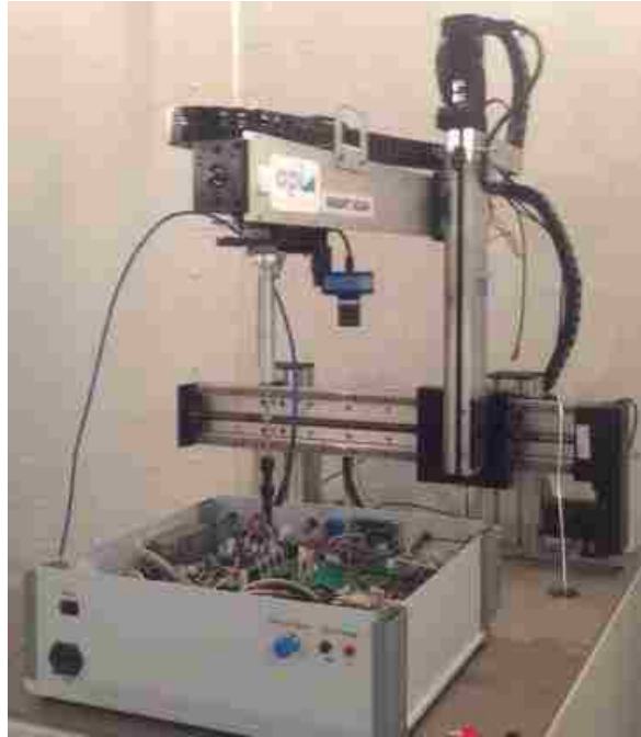
Figure 1.1. Robotic near field scanning system from API
