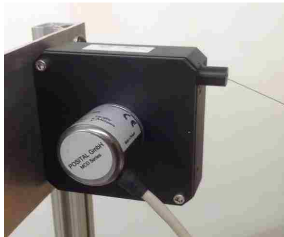
Figure 2.3. Draw wire sensor
