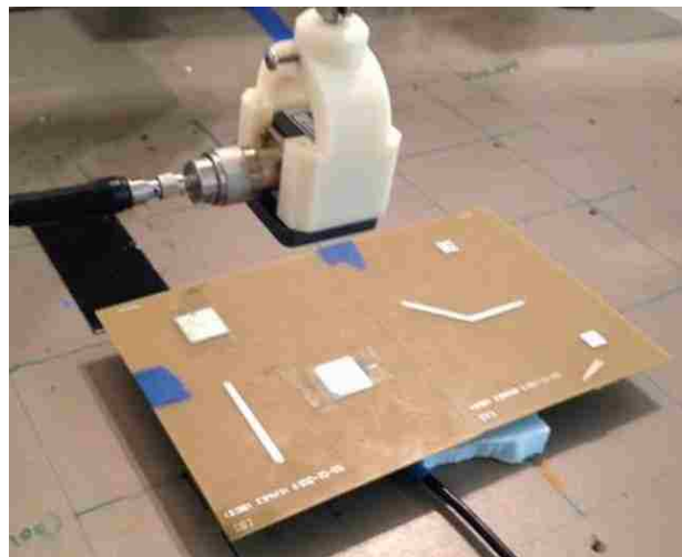
Figure 4.10. Custom board with a waveguide above
