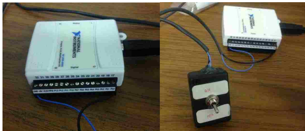
Figure 2.36. A switch implemented through DAQ for pausing scanning
