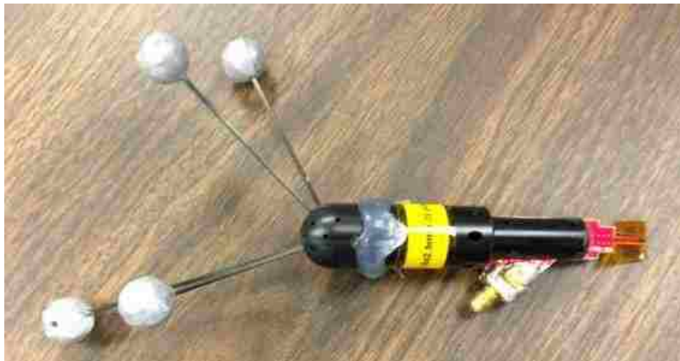
Figure 2.47. Field probe with rigid body fixed on top of it.
