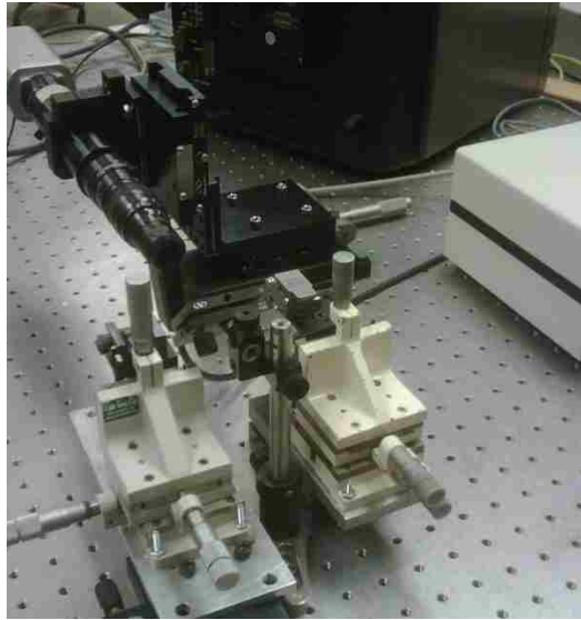
Figure 3.6. Picture of the backward coupling efficiency evaluation experiment
