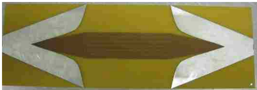
Figure 3.2. The Second Layer of the TEM Cell Septum
