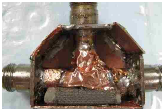
Figure 2.48. Photo of 6 dB Splitter
