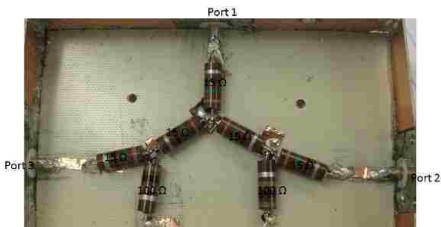
Figure 2.49. Photo of the 10-dB Splitter
