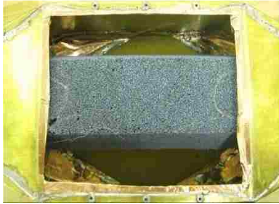
Figure 3.6. Photo of Cell from Bottom with Absorbing Material Added
