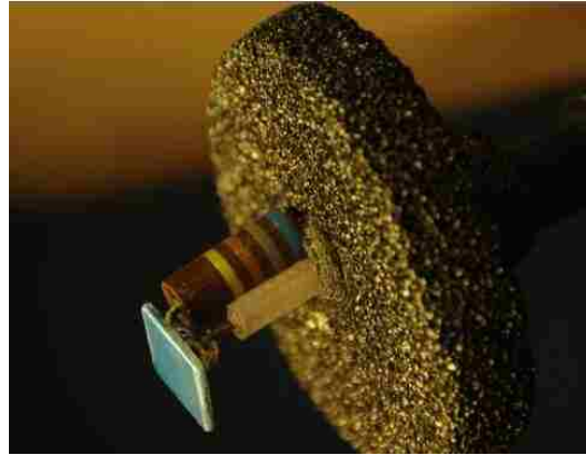
Figure 2.2. Photo of the E-field Probe
