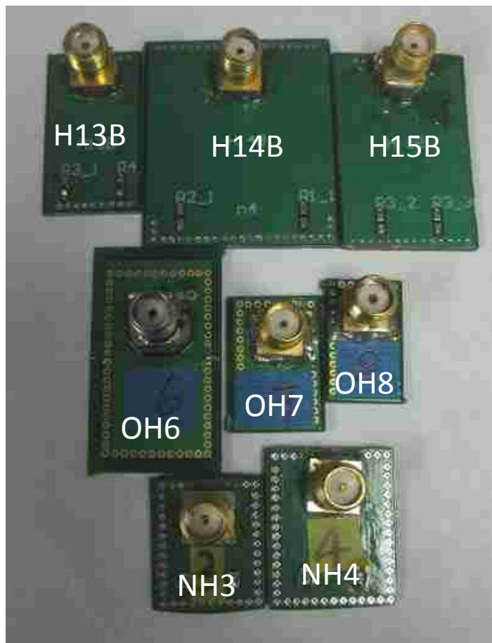
Figure 2.16. The Photo of the H-field Probes
