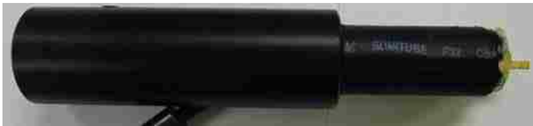
Figure 2.35. Photo of the Reference H-field Probe
