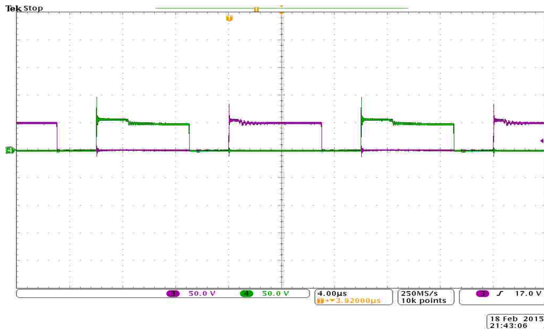
Figure 4.3. Voltage of drain to source with Si based MOSFET
