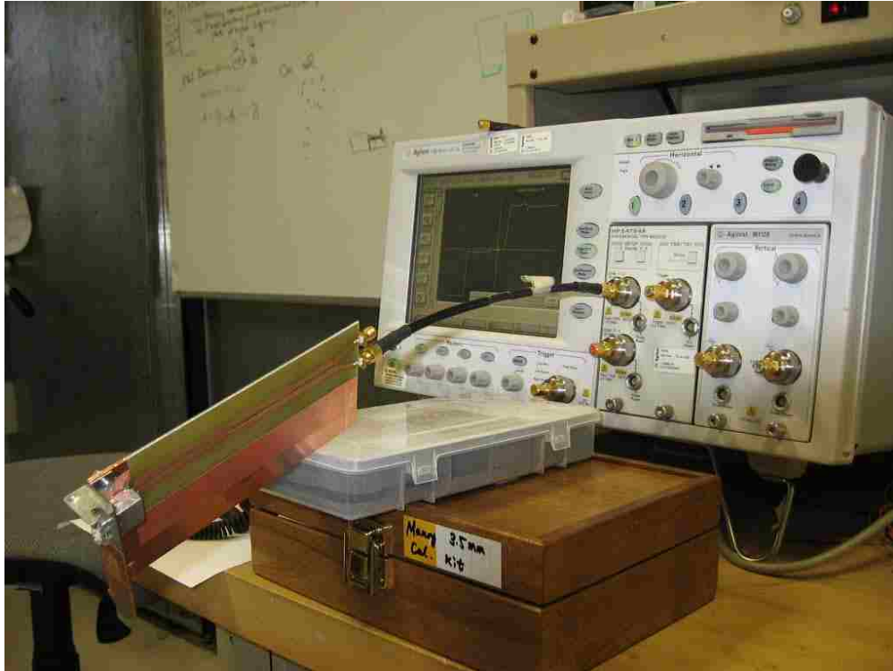
Figure 2.4. TDR Test Setup for Single Trace on the PCB
