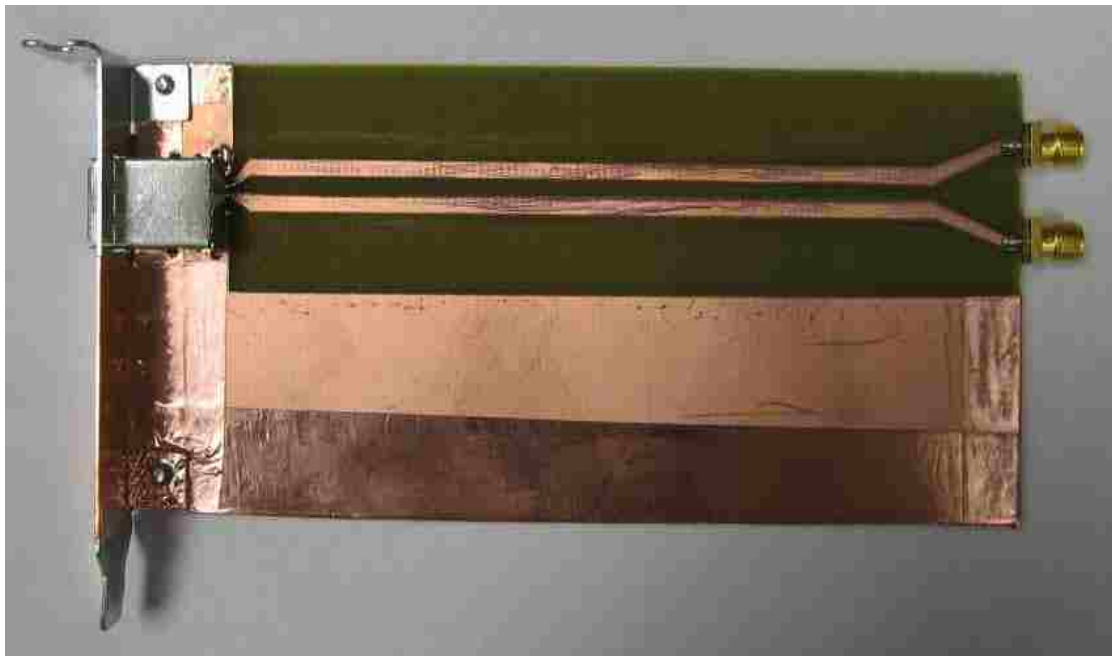
Figure 2.3. 2-Layer PCB with Differential Signal Traces and with Connectors Mounted
