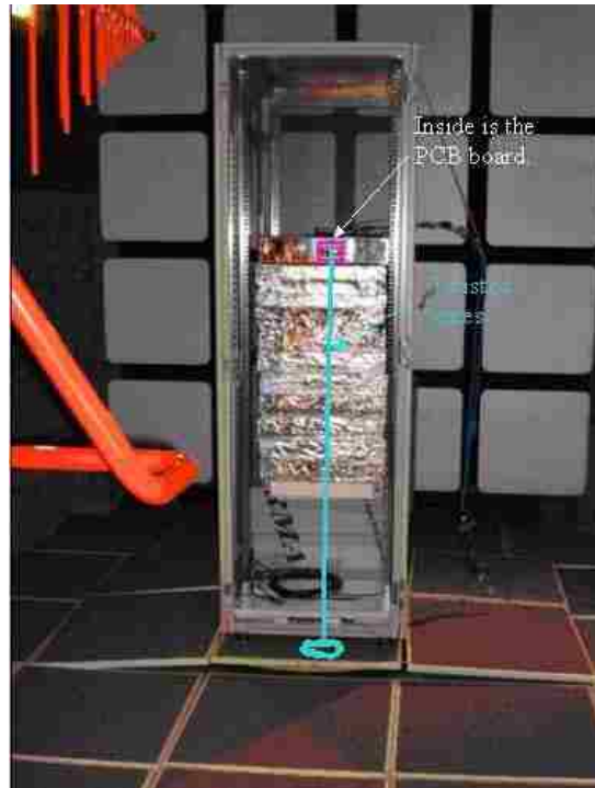
Figure 2.17. Cabinet Setup for Three-Port Mixed-Mode S-Parameter Measurements
