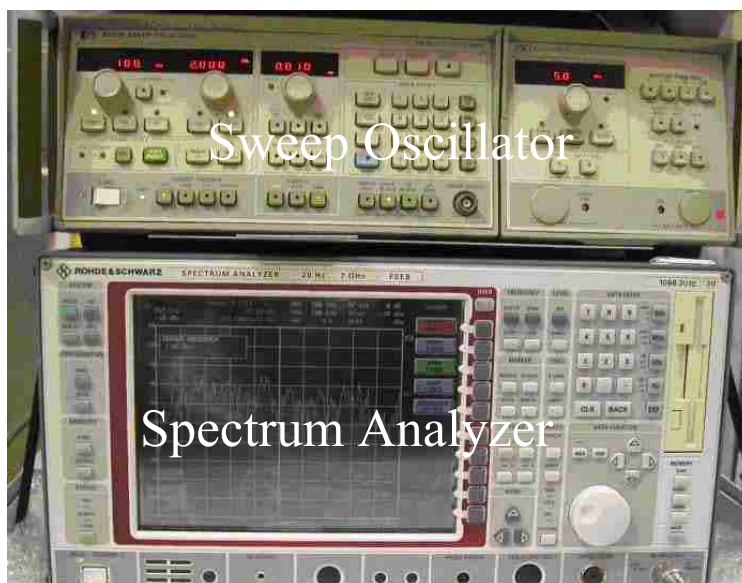
Figure 2.10. Spectrum Analyzer and Sweep Oscillator for S 21 Measurements of Cabinet
