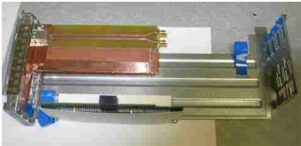
Figure 2.7. The PCB Inserted into a Slot of a Module in the Computer Node
