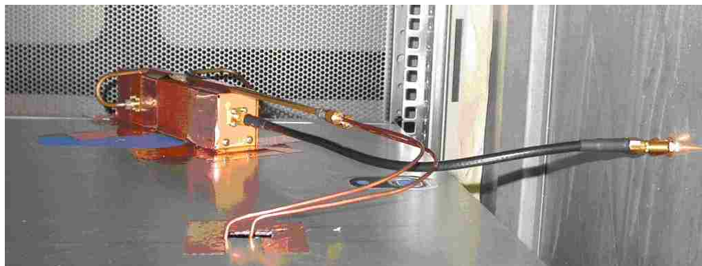
Figure 2.11. Hybrid Setup in Spectrum Analyzer or 2-port VNA Measurements
