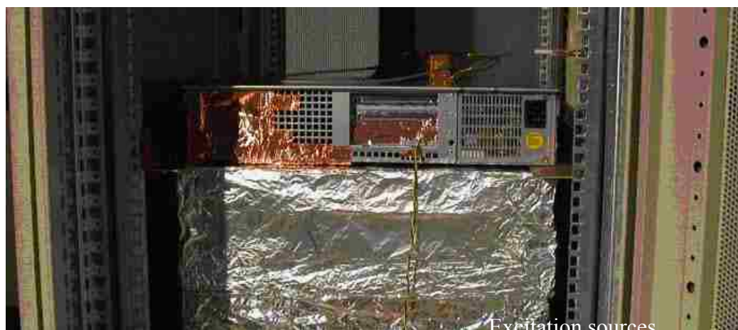
Figure 2.8. Two Twisted Wires as the Radiation Source in the S-parameter Measurements
