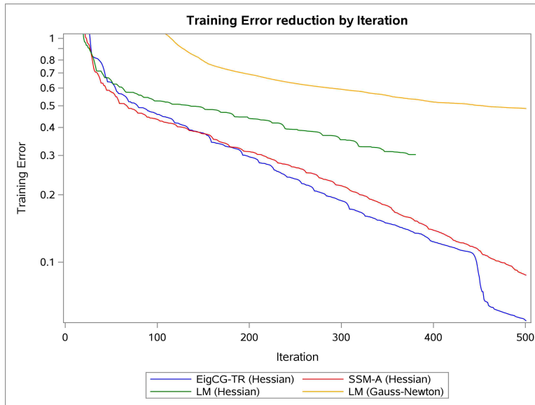
Figure 5.4: Training loss on each iteration of EigCG-TR, SSM-A, Levenberg-Marquardt (Hessian and Gauss-Newton)
