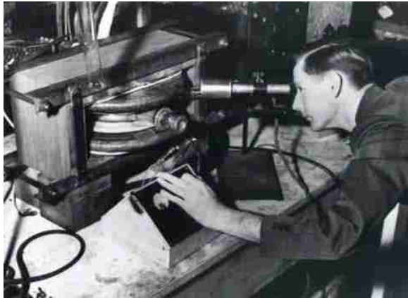
Figure 2.15: Donald Krest with his invention the first ever betatron. The betatron was developed at the University of Illinois and was a 20 MeV machine.[39]
