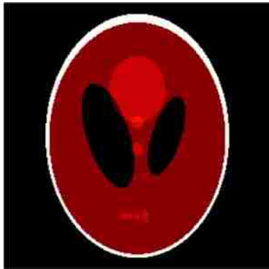
Figure 2.5: The Shepp-Logan phantom depicted here is used as a standard for tomographic reconstruction algorithms.
