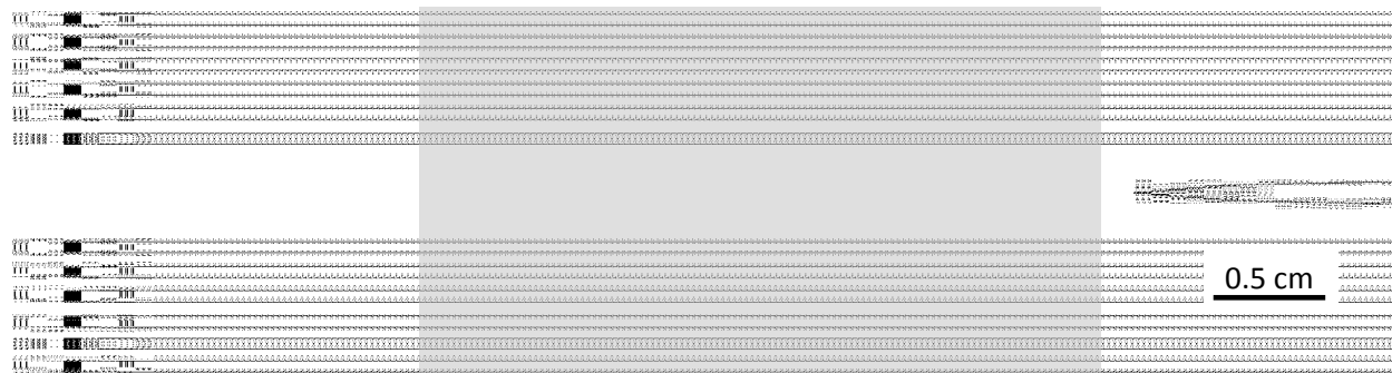
Figure 5.1 AutoCAD 2008 rendering of a microfluidic device that can provide high throughput micro-sampling (HTMSU). The device used a series of microchannels that were decorated with antibodies specific for the target cell. The antibodies were immobilized beneath the gray shaded region, which consisted of 37 straight microchannels that were uniformly 3 cm long and 30 \mu\text{m} wide. The entire device was 150 \mu\text{m} deep. The output end contained a conductivity sensor that consisted of a pair of Pt wires placed orthogonal to the fluid flow path.
