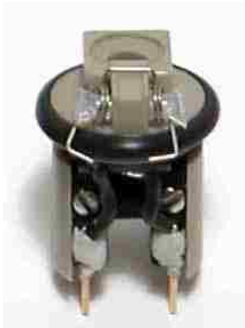
Figure F.1 Nose cone assembly for tapping mode AFM.
