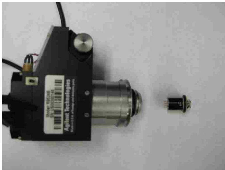
Figure E.1 Scanner and nose cone assembly for current sensing AFM. The nose cone for current sensing has four pins.
