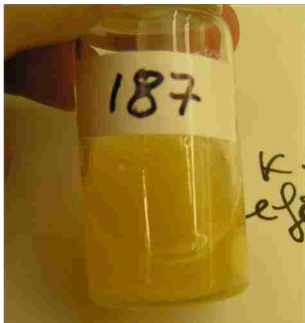
BMIMAc and chitosan before heating to 85-95°C
