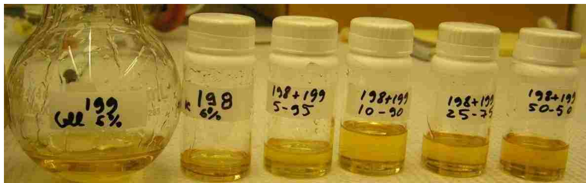
Figure 5.3 Polymeric solutions containing chitosan and/or cellulose dissolved in BMIMAc.
