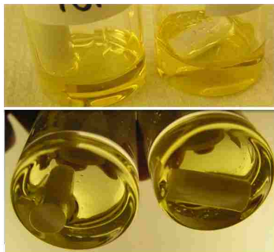
BMIMAc and chitosan after heating to 85-95°C (a homogeneous transparent solution)
