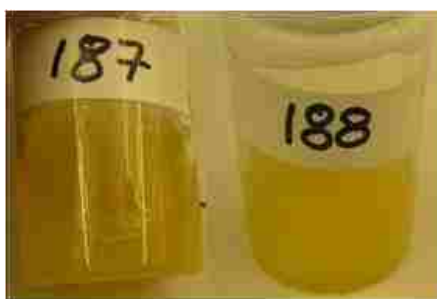
Figure 5.2 Slurries of chitosan (187) and cellulose (188) in BMIMAc before dissolution.
