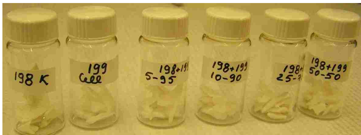
Figure 5.5 Polymeric films containing chitosan and/or cellulose obtained by freeze drying technique.
