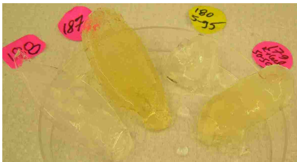
Figure 5.4 Polymeric films before freeze drying (from left to right: cellulose film, chitosan film, chitosan 5 wt%-cellulose 95 wt% film, and chitosan 50 wt%-cellulose 50 wt% film).
