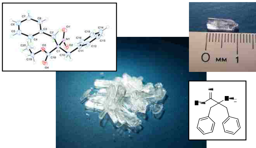
Figure 8.1. Single crystals of ethyl 2-benzyl-2-nitro-3-phenylpropanoate which were synthesized by the dialkylation on the alpha carbon of ethyl nitroacetate with benzyl bromide under basic conditions (adapted from McCandless, G. T. Thesis, Louisiana State University, 2008). 1
