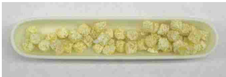
Figure 7.1. Mixtures of bioceramic and polymeric materials are converted to a slurry, mixed with polyurethane foam, and then annealed to produce a porous material. The scaffolded product (prior to annealing) is shown in a boat-shaped alumina crucible.
