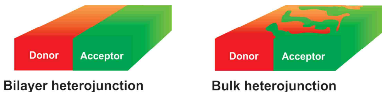
Figure 2.1. Schematic diagrams of heterojunction type organic solar cells.
