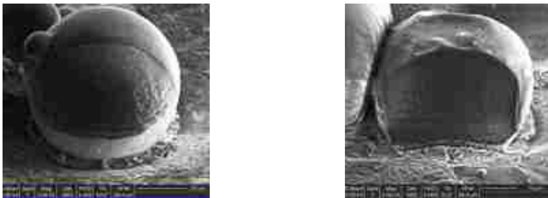
Figure 1.6 External surface of a ChemMatrix bead (left) and section of a ChemMatrix bead (right) by Focused Ion Beam (FIB).
