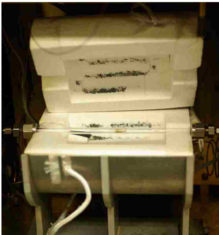
Figure 2.4 Fused silica flow reactor located in the high temperature furnace
