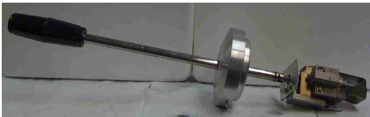
Appendix Figure F Carbon gun attached to the gun extraction rod.
