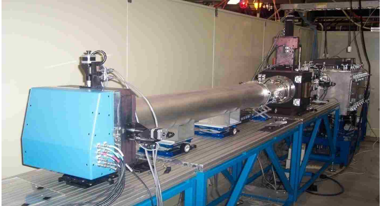
Figure 2-3 Picture of the SAXS endstation. The blue box on the left is the detector. The pinholes are obscured by the black sample chamber and grazing incidence-small angle x-ray scattering “coffin” in the background on the right side of the picture.
