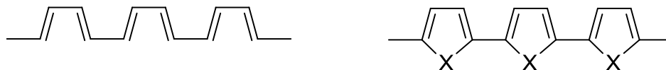
Figure 3-2: Structure of cis -(CH) x and heterocyclic conjugated polymers stabilized by a heteratom
