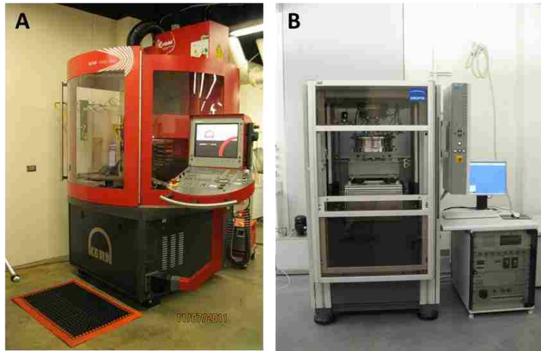
Figure 1.4 (A) Kern micromilling machine (MMP) is a computer numerically controlled (CNC) milling machine that is used to pattern microstructures on metal mold inserts using very small milling bits (down to 25 \mu\text{m} diameter) rotated at very high speeds in the range of 40,000 – 200,000 rpm. Mold inserts can then be used as masters for the production of microstructures on polymer substrates (B) Hex03 hot embossing equipment capable of molding polymer parts containing features with micro- and nano-dimensions including high aspect ratios (>10 : 1) through a combination of heat and pressure. It is commonly used to produce polymer microfluidic chips for biomedical applications.
