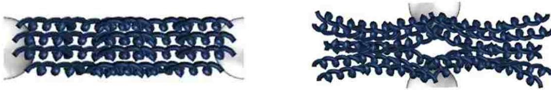
Figure 3.20 Schematic representation of possible arrangements of PBLG chain attached to the silica surface.
