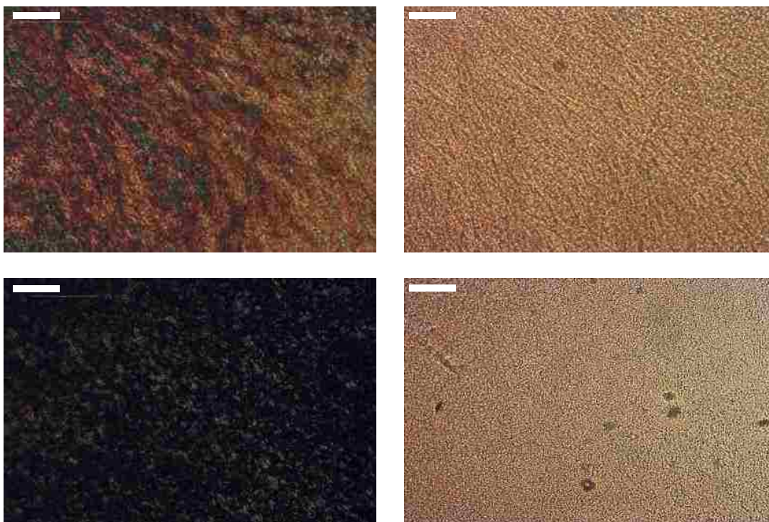
Figure A3.3 Composition: 23.0 wt% PBLG, 22.6 wt% silica, 54.4 wt% pyridine. (MC.1.41F) Photograph on the right is the same spot in the sample as on the left, but without crossed polarizers. Scale bar is 100 microns.
