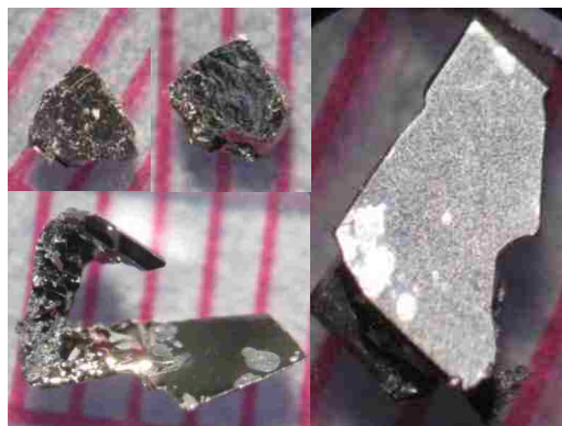
Figure 3.1 Image of un-etched single crystals retrieved from Al flux (grey spots on surface). Two upper left images show the more block-like morphology of the single crystals of \text{CeM}_2 , with the lower left and right image depicting the blade morphology of \text{GdM}_2 single crystals. Each graduation marks 1 mm.
