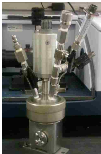
Figure 3.7 SpectraTech High Pressure In-Situ Circle Reaction FT-IR Cell
