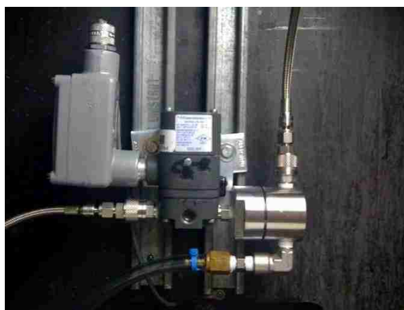
Figure 3.6. The Mass Flow Controller (left) and the I/P-Back Pressure Regulator (right).
