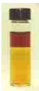
Figure 2.1. A vial of the hydroformylation reaction solution when using an acetone/water solvent, causing the biphasic system.
