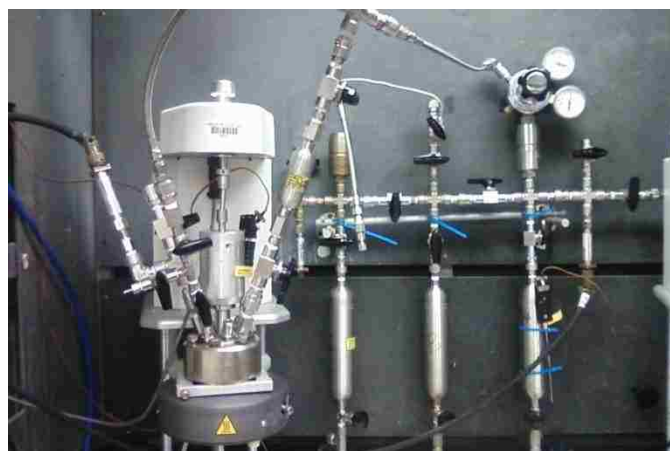
Figure 3.3. Assembled Autoclave Mark II Reactor and Gas Reservoir System
