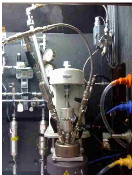
Figure 3.5. Flow-control Autoclave Reactor design
