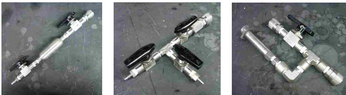
Figure 3.2. Autoclave Mark II Reactor arms: Olefin Pressure Injection Arm (left), Sampling Arm (middle), and Purge Arm with Pressure Transducer (right).
