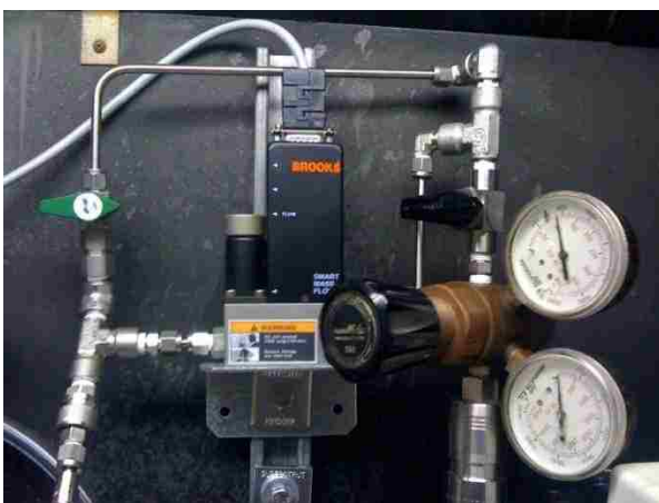
Figure 3.6. The Mass Flow Controller (left) and the I/P-Back Pressure Regulator (right).
