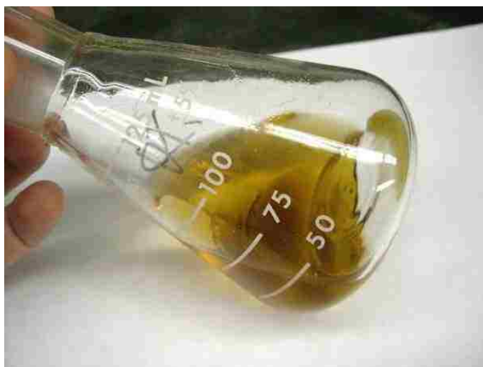
Figure 5.4. Catalyst after hydroformylation.
