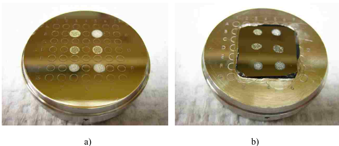
Figure 2-9. Photographs of 7x7 Omniflex MALDI targets; a) a stainless steel and b) a target modified to accommodate a silicon wafer. A 0.5 \mu\text{L} quantity of analyte mixed with 1 \mu\text{L} of matrix was deposited on both target substrates and allowed to air dry. First row: CHCA and SA; Second row: peptide calibration standard with CHCA; Third row: BSA with SA.
