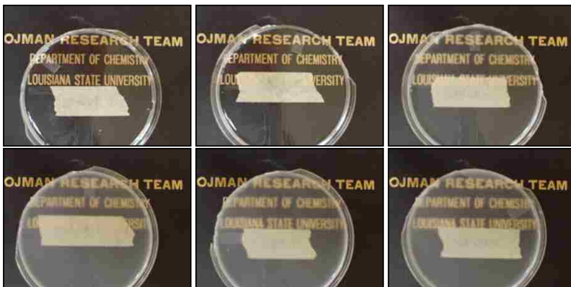
Figure 3-31: Optical clarity of the films containing various concentrations of Lauryl Acrylate. From left to right and then top to bottom the lauryl acrylate concentration was 8.6, 16.5, 23.0, 28.6, 33.0, and 37.7 mol%.
