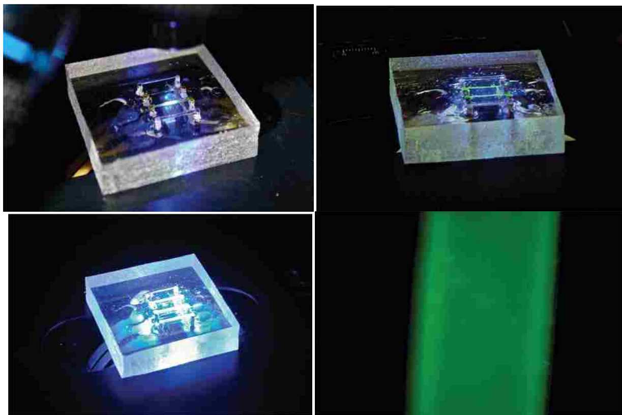
Figure 3-39: Fluorescent images of PETA-co-TMPTMP microfluidic devices containing an aqueous fluorescein isothiocyanate (FITC) solution. Photographic images of microchannels containing the FITC solution are shown on top and bottom left and top right, and a fluorescent microscopy image is shown on the bottom right.
