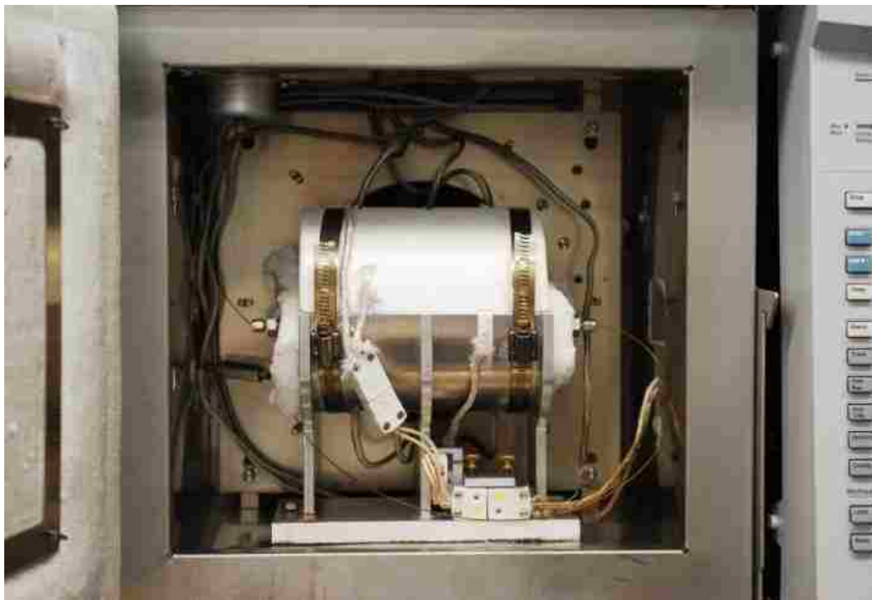
Figure 2.1 Omega Furnace that Houses the Flow Reactor inside the Thermal Reactor Compartment
