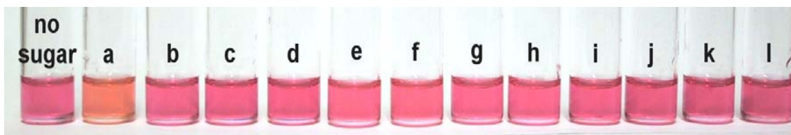
Figure 2.6. A selective solution color change is observed for D-fructose when added to colored solutions of 2.8 and 2.9 : (a) D-fructose, (b) D-glucose, (c) D-psicose, (d) D-allose, (e) D-ribose, (f) D-xylose, (g) D-trehalose, (h) melezitose, (i) D-turanose, (j) D-maltose, (k) sucrose, (l) D-raffinose. Sugars in vials labeled a, b and g-l are found in honey.
