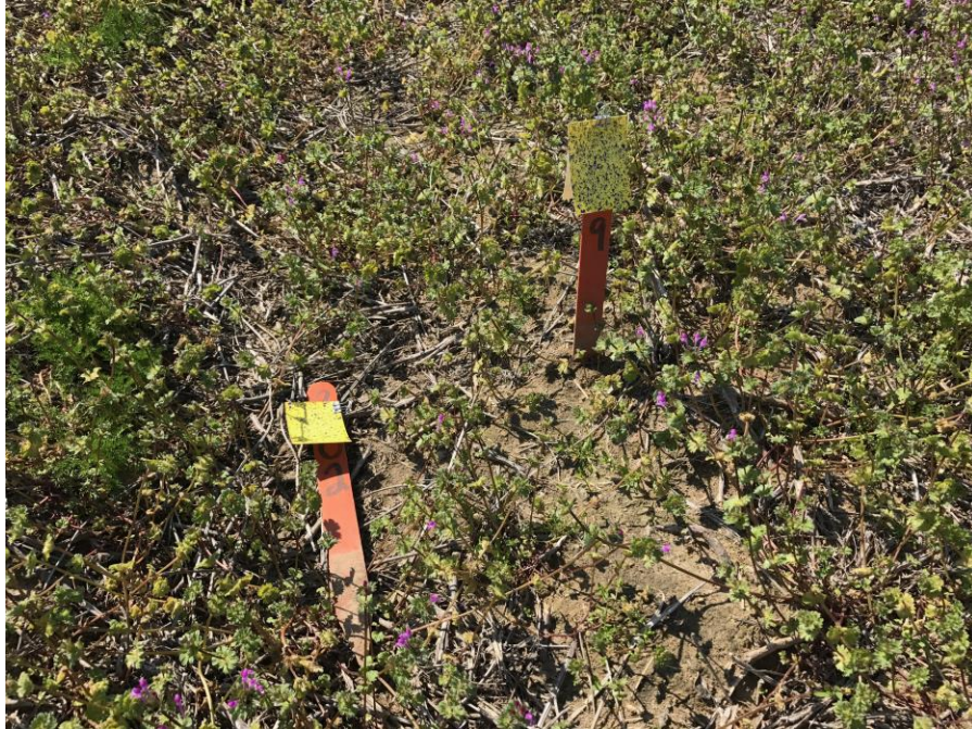
Figure 6. Water sensitive spray cards were used to capture percent coverage readings of liquid carried sprays.
