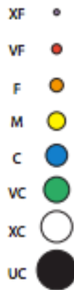
Figure 2. The complete spectrum of droplet sizes arranged from smallest to largest: Extra Fine(XF), Very Fine(VF), Fine(F), Medium(M), Coarse(C), Very Coarse(VC), Extra Course(XC), Ultra Course(UC). TeeJet Technologies. (2016a). Catalogs and Bulletins . Retrieved January 2017, from TeeJet: http://www.teejet.com/literature_pdfs/bulletins/B124_Spray_Nozzle_Rate_Droplet_Size_Chart_20-inch.pdf
