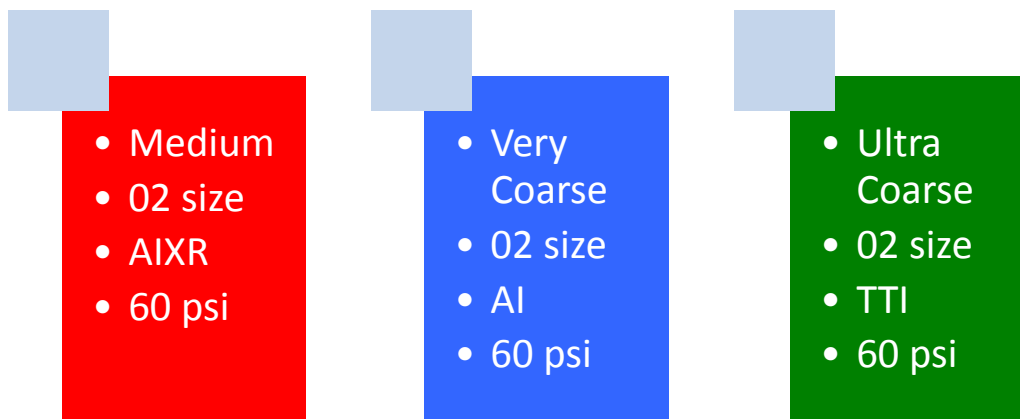
Figure 7. Boom setup for all passes sprayed at the 11 km/h (7 mph) travel speed. Spraying section widths were 6 m (20 ft.) with 3 m (10 ft.) unsprayed between each section
