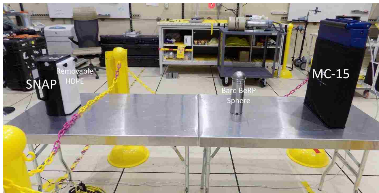
Figure 3.1: Bare BeRP Ball experiment with optional polyethylene shield attached to the SNAP detector.
