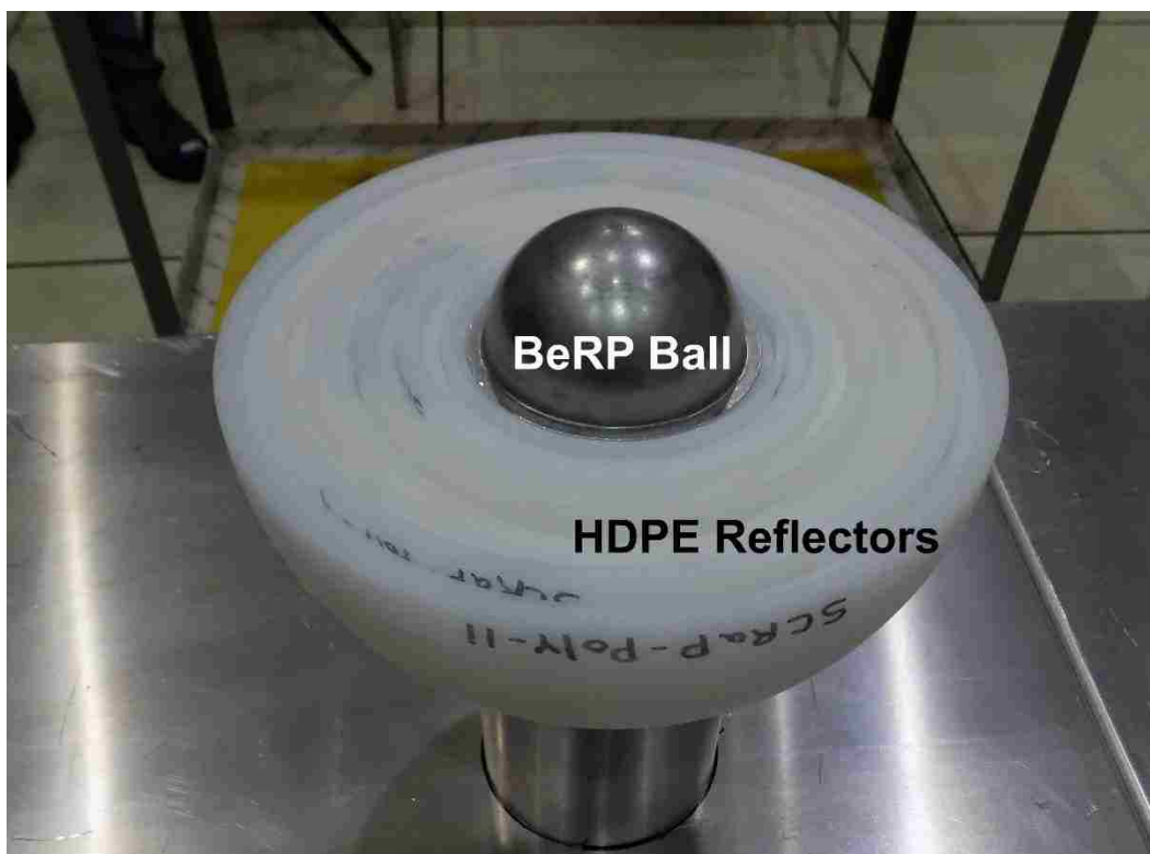
Figure 3.2: BeRP ball in the lower half of the HDPE reflector.
