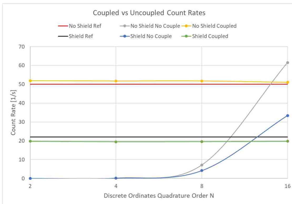
Figure 6.13: Coupled vs Uncoupled SNAP Count Rates with and without HDPE Shield.
