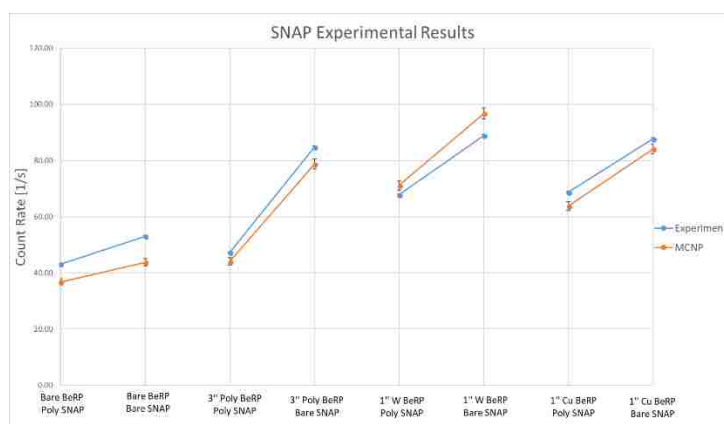
Figure 4.2: MCNP vs Experimental Count Rates for SNAP detector.
